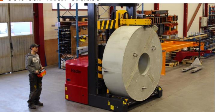
Coil Car with Cradle offers an easy solution to the transportation of coils, with capacities up to 55,000 lbs. and custom larger options available. Ultimately eliminating the need for an overhead crane or railbased systems. As an all-electric battery powered unit, the Coil Car operates independently from the rest of your production line—allowing the operator to use it whenever and wherever necessary.
