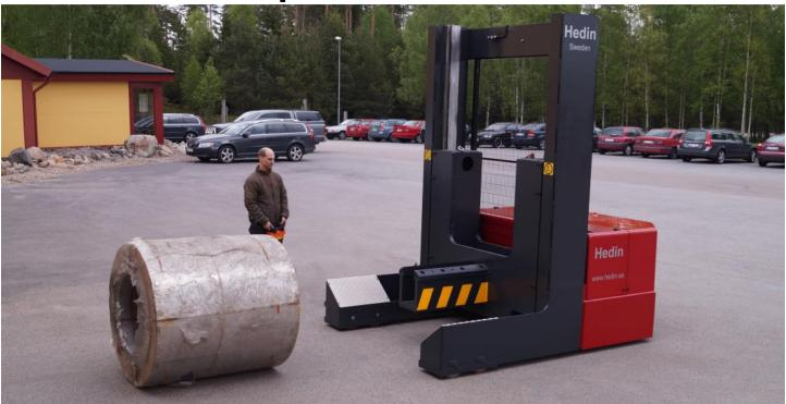
Coil Car with Spike offers an easy solution to the transportation of coils, with capacities up to 55,000 lbs. and custom larger options available. Ultimately eliminating the need for an overhead crane or railbased systems. As an all-electric battery powered unit, the Coil Car operates independently from the rest of your production line—allowing the operator to use it whenever and wherever necessary.
