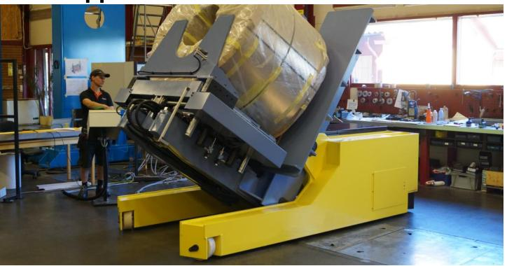
Coil Tippers are an all in one solution for the positioning of coils. We offer the ability to tilt 90° horizontally and vertically, and an added function of 180° rotation. With capacities up to 100,000 lbs., our Coil Car offers an easy solution to the transportation of coils, ultimately eliminating the need for an overhead crane or rail-based systems.
