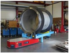
**High Capacity** GT Tuggers have capacities that can move loads up to 220,000 lbs., making even the heaviest moves possible.
