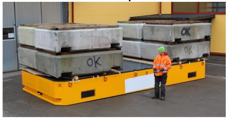
Mutli-Drive Flatbed Transporters makes moving heavy loads easy, with operating capacity up to 1,000,000lbs. The Flatbed Transporter multi-drive offers a zero-degree turn radius and is controllable via radio controller or an optional automated guidance system for precise automated movement. Our Multi-Drive Flatbed Transporters can also be configured to operate in tandem, enabling the movement of loads up to 2,000,000lbs.
