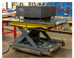
Lift with Extended Bolt-on Tops Above shows our oversized table top that bolts on to the lift table. Our Extended Tops are built to your measurements.
