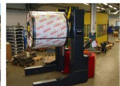
**Adjustable Coil Height** The adjustable stroke allows for variable height changes, giving operators the freedom to easily and efficiently position coils.
