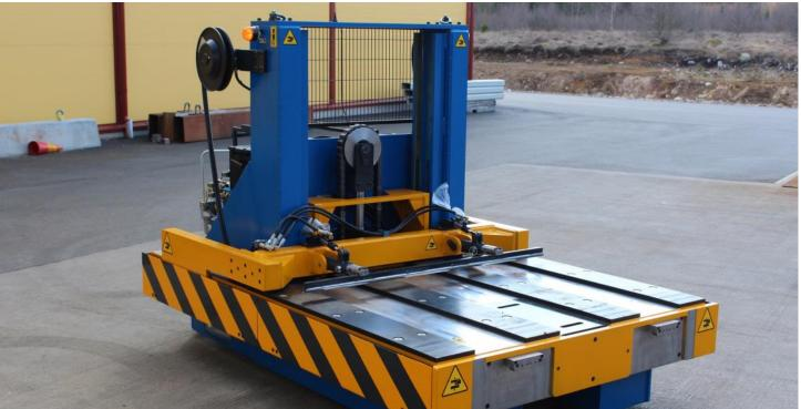
The Mold & Die Transporter is designed to maximize safety and efficiency, creating the easiest way to transport and change dies. With capacities up to 200,000 lbs., the Mold & Die Transporter allows operators to move heavy dies via remote control from a safe distance - improving efficiency and reducing time lost between die changes.
