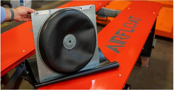
Airfloat Air Casters are pneumatic devices that form a lubricating film of air between the load and floor surface, similar to that of a hovercraft or an air hockey table. These are a great solution for moving and positioning heavy and difficult loads with low friction, omnidirectional movement. Designed with slide-out trays, our casters are able to be serviced without having to remove the load.
