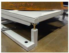
Adjustable Leveling Pads Upenders adjustable leveling pads for leveling the upender's deck in the 0° and 90° positions.
