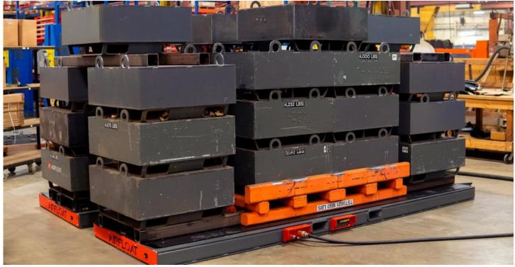
Air Plank systems allow for the safe, nearly frictionless movement of large loads or machinery. Steel Air Planks are available in capacities up to 204,000 lbs. per set of two planks, and are available in lengths up to 180 inches. Manufactured from structural steel, these planks are durable, heavy-duty and built for years of trouble-free operation.
