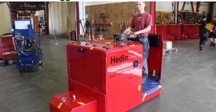
The Ride-On Tug is designed to distribute loads up to 132,500 lbs. to the wheels, allowing an operator to ride on board and confidently steer the load. Featuring a rechargeable battery and speeds up to 150 fpm, the Ride-On tug is ideal for moving loads around your facility in a quick, safe, and controllable manner.
