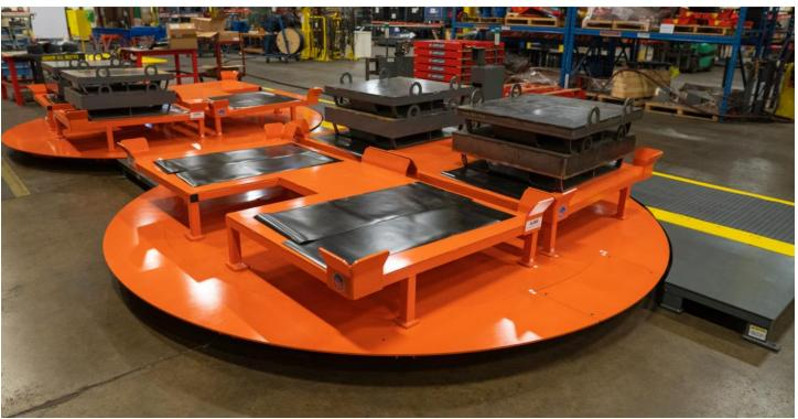
Air Caster Turntables are fitted with Airfloat air caster technology. Which creates a thin layer of air between the base and the top of the table, making the table nearly friction-free to move loads effortlessly. Quality materials matter, as reflected by our 100% urethane diaphragm design in our air casters for superior wear resistance.
