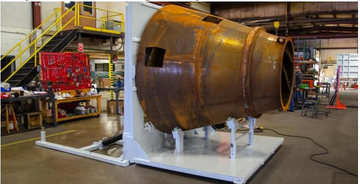
Prioritize worker safety by eliminating dangerous overhead crane maneuvers by using 90° Upenders in your assembly or fabrication operation. The Upenders are designed to flip heavy or large objects 90° to optimize your product's fabrication or assembly with the push of a button. Upenders not only offer a safe way to flip products, but they also save substantial time over other methods.
