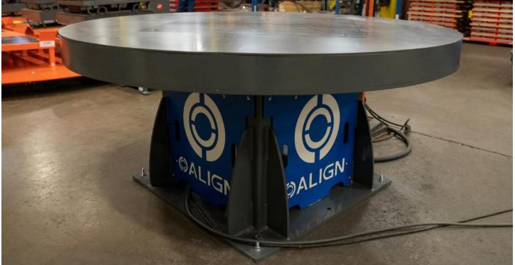
Maximize efficiency in your robotic cell with the Precision Mechanical Turntable. The table is accurate up to 0.01" and boasts a weight capacity up to 5,000 lbs. It can be easily integrated into existing or future work cells thanks to its compatibility with all major robotic controllers. Customizable round and rectangular tops are available from 60" up to 120".
