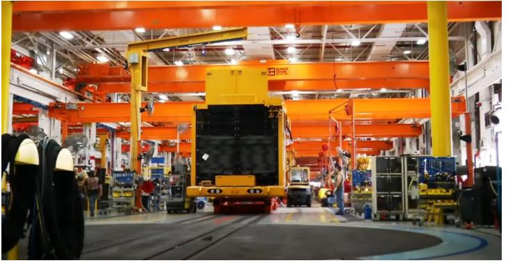
Flush Floor Air Caster Turntables package our popular Air Caster Turntable into a solution designed for operations needing turntables to interact with fork lifts or rail systems. Our flush floor systems are more practical than mechanical ones, with a capacity of 100,000 lbs, max top size of 324", and optional rail spurs and curb ring.
