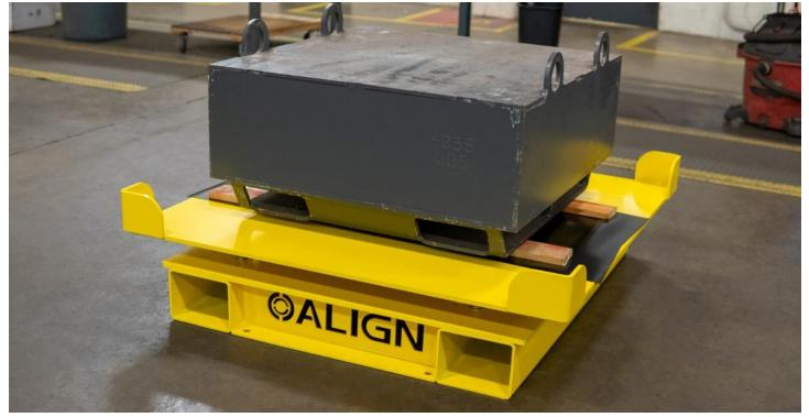
Both of Align's Mechanical Rotate options allow for you to easily rotate parts containers or other heavy loads. Offering bolt-on or stand-alone operation, our rotates use sealed, lubricated-for-life slewing bearings or turntable bearings with cam follower supports. Options include pneumatic friction brakes, 90 and 180-degree spring lock pin, riser base with fork pockets and corner locators to hold the container in place.
