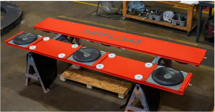
Air Plank systems allow for the safe, nearly frictionless movement of large loads or machinery. Aluminum Air Planks are available in capacities up to 75,000 lbs. per set of two planks, and are available in lengths up to 144 inches. Manufactured from extruded aluminum, these planks are durable, lightweight and built for years of trouble-free operation.
