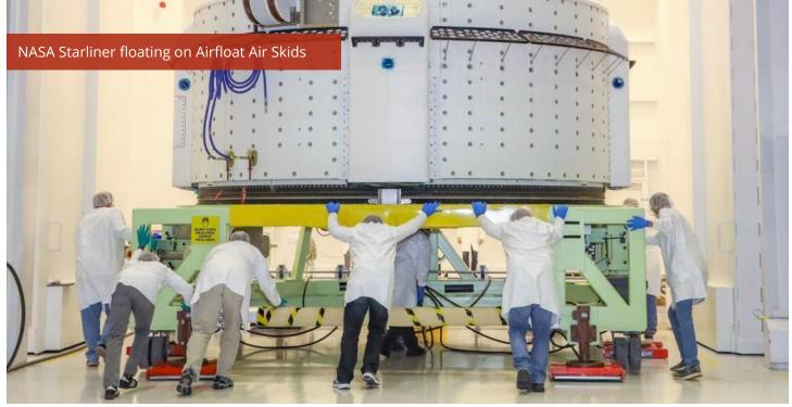
Air Skid systems allow for the safe, nearly frictionless movement of large loads or machinery. Air Skids come in a variety of sizes, and are durable and lightweight - built for years of trouble-free operation. Easily move heavy loads by utilizing air caster technology to move 1,000 lbs. with approximately 1 lbs. of force.
