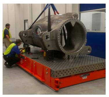
**CMM Air Caster Transporter** Guided Air Caster Transporter with CMM Pallet System designed for Mining Truck Manufacturer.
