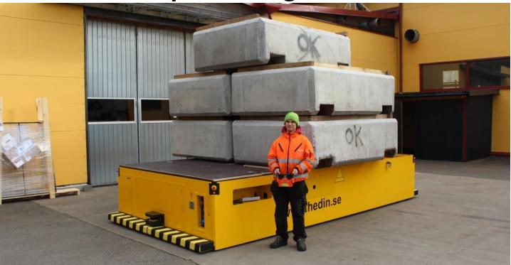
Designed to move loads up to 220,000 lbs. with a battery propelled drive unit, the Flatbed Transporter makes moving heavy loads on a facility floor easy. The Flatbed Transporter offers controls via radio controller or an optional automated guidance system.
