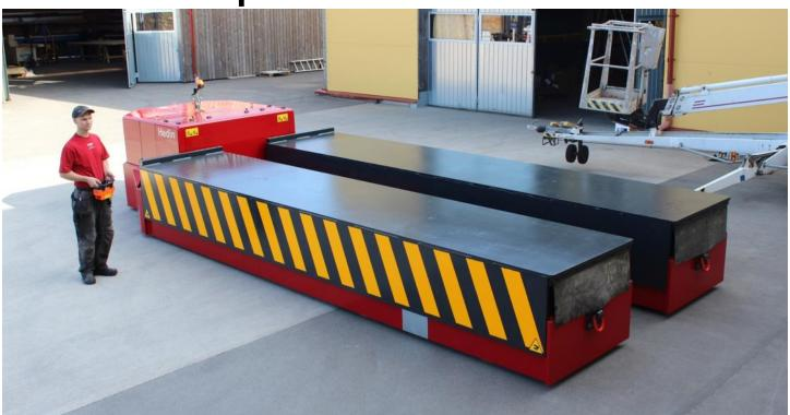
The Pallet Transporter is the ideal solution for easily moving heavy loads on steel pallets, with capacity of up to 132,500 lbs. The Pallet Transporter is available with a number of options including safety scanners, enhanced batteries, and AGV drive systems.
