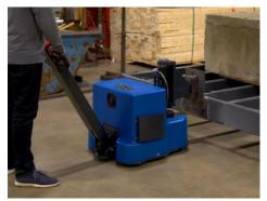
**30,000 lbs. Capacity** APS030-1200 features a hitch point capacity of 6,750 lbs, 45 minute battery life, 5,500 ft-lbs. of torque, and movement speeds of 120 fpm.
