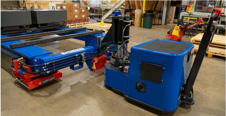
Move up to 120,000 lbs. using a single operator with The Ox Power Tugger. The Power Tugger enables a single operator to move and position heavy weight pallets and loads on wheels, and can comfortably move up to 120 feet-per-minute. Designed to lift the front end of non-motorized trailers or pallets, distributing the load to the wheels on the trailer.
