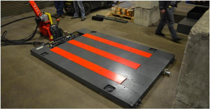
Air Caster Platforms allow an operator to efficiently move pallets or any heavy or difficult to handle load up to 120,000 lbs. with ease. Using Air Caster technology, Air Platforms provide near friction-free movement in any direction, giving them an advantage over wheeled carts and forklifts for moving pallets and heavy loads. Pair with Pneumatic Tugger for fully air powered single man movement.
