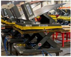
Lift with Pneumatic Tilt Featured above is our Pneumatic Lift Table combined with our Tilt Table. This is often used for part packaging or presentation.
