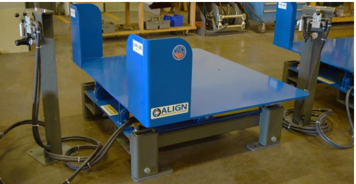
Pneumatic tilt tables are designed to be stand-alone or bolt-on configurations with other equipment like our pneumatic lift and mechanical rotates. Safety features include two up-stop chains per actuator, a safety prop for maintenance, corner retainer, safety skirt, and enclosed base pan to protect internal components.
