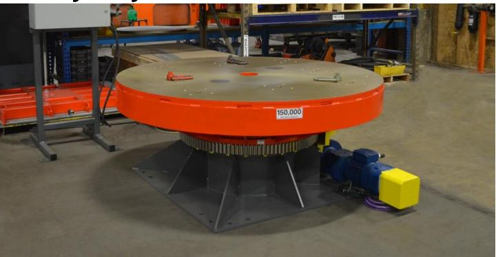
Heavy Duty Mechanical Turntable features a geared slewing bearing allowing for high weight capacities up to 150,000 lbs, standard sizes from 48" to 120" and the ability to run extended amounts of time. Custom top sizes are available, and if needed, with larger load sizes, wheels will be added in order to give the table additional stability. These turntables are also excellent for outdoor areas or areas that an air supply cannot be easily connected.
