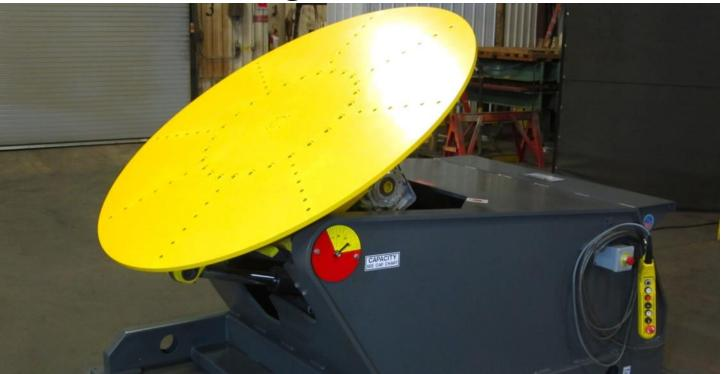
Simplify circular welds and improve worker ergonomics with our Two Axis Welding Positioners - designed for maximizing stability, reducing vibrations, and preventing elastic deformations that may compromise weld quality. Our positioners feature a 115° incline, weight capacities up to 25,000 lbs., and have face diameters up to 76 inches.
