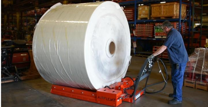
Fixed and adjustable fork style roll transporters allow for rolls to be lifted right off the floor without needing forklifts or overhead cranes. Featuring up to 2" of stroke and omni-directional nearly friction-free movement with air casters. Easily maintain the equipment with slide-out air caster trays that can be serviced without removing the load.
