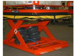
Lift with Mechanical Rotate Putting our Pneumatic Lift Table with our Mechanical Rotate makes for easy rotation of the table top. Interactive PDF
