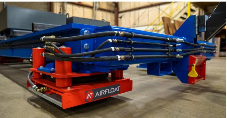
Lift Glide Air Skids are designed to be retrofitted to existing wheeled units, allowing you to utilize existing equipment and switch to air caster technology when the load becomes too heavy to push. Compression springs keep the Lift Glide Air Skids retracted off the floor, and when engaged, the air skid extends down to lift the wheels off the floor and float the unit.
