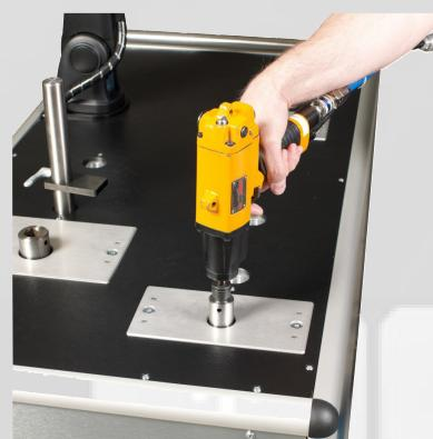
The tJRS Opta is the only fully automated Joint Simulator Bench that is based on a threaded fastener. This means that Joint conditions can be set up in the same way as in real fastener applications, and also the Joint can be automatically “backed off”. As a result, Tools can be tested off-line under the most realistic conditions of any automated Joint Simulator, in a quick and efficient manner.
