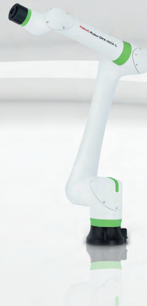
CRX-20iA/L Payload: 20 kg Reach: 1,418 mm
