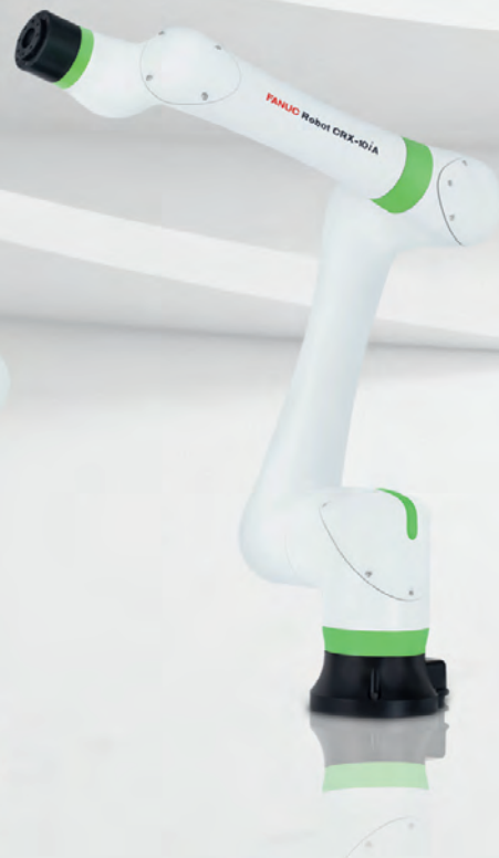
CRX-10iA Payload: 10 kg Reach: 1,249 mm
